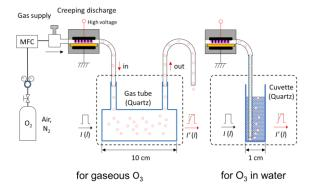
Fig. 1: Schematic of the experimental set-ups to monitor the gas phase O<sub>3</sub> (lhs) and O<sub>3</sub> in water (rhs).
