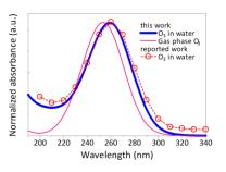
**Fig. 2**: UV absorption spectra of gaseous  $O_3$  and dissolved  $O_3$  in water with a reported spectrum.
