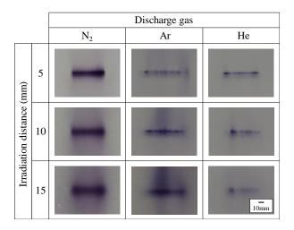
Fig.3. Irradiation shapes of line type atmospheric pressure plasma jets
