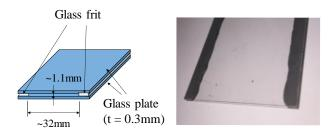
Fig.1. Structure and photograph of rectangular tube
